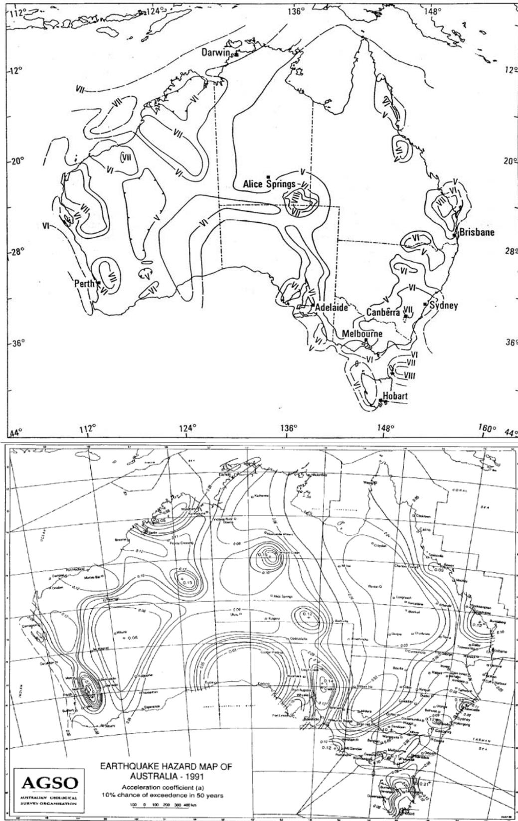
**Figure A2 - Two hazard maps for Australia: A (top) from Gaull et al (1990) shows intensity hazard with 475 year return period; B (bottom) is PGA for the same return period. A was produced before the Tenant Creek earthquakes in Northern Territory; B after it.**
