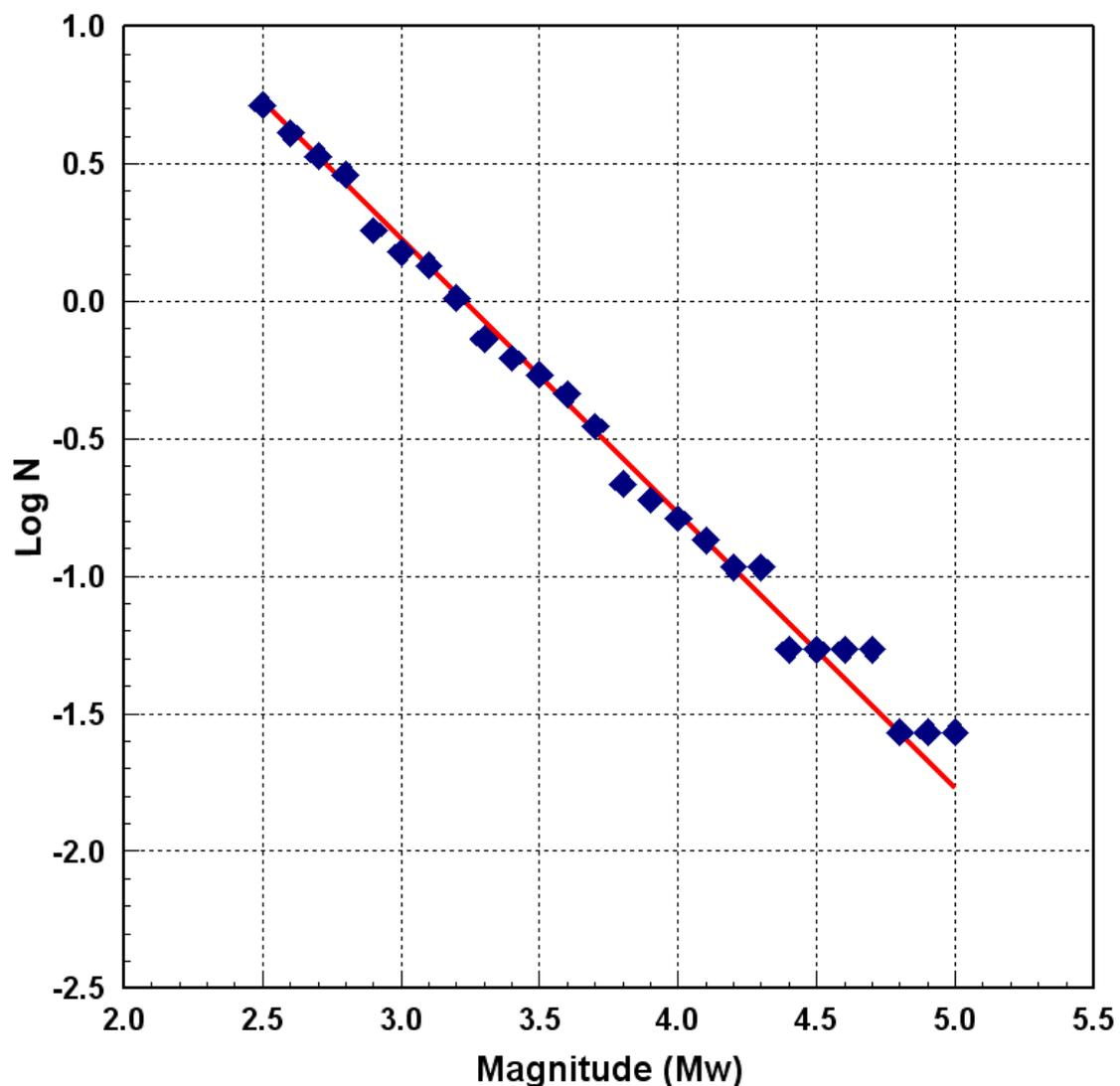
Figure 12 - Gutenberg-Richter plot for post 1970 UK seismicity. The red line shows Equation (1).
