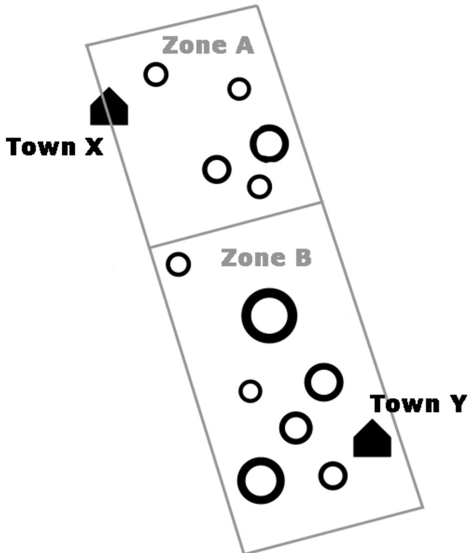
**Figure A1 - Hypothetical illustration of a typical problem in source zonation: are Zones A and B to be kept separate or merged? The decision taken has different effects on the conservatism of the hazard at X and Y.**
