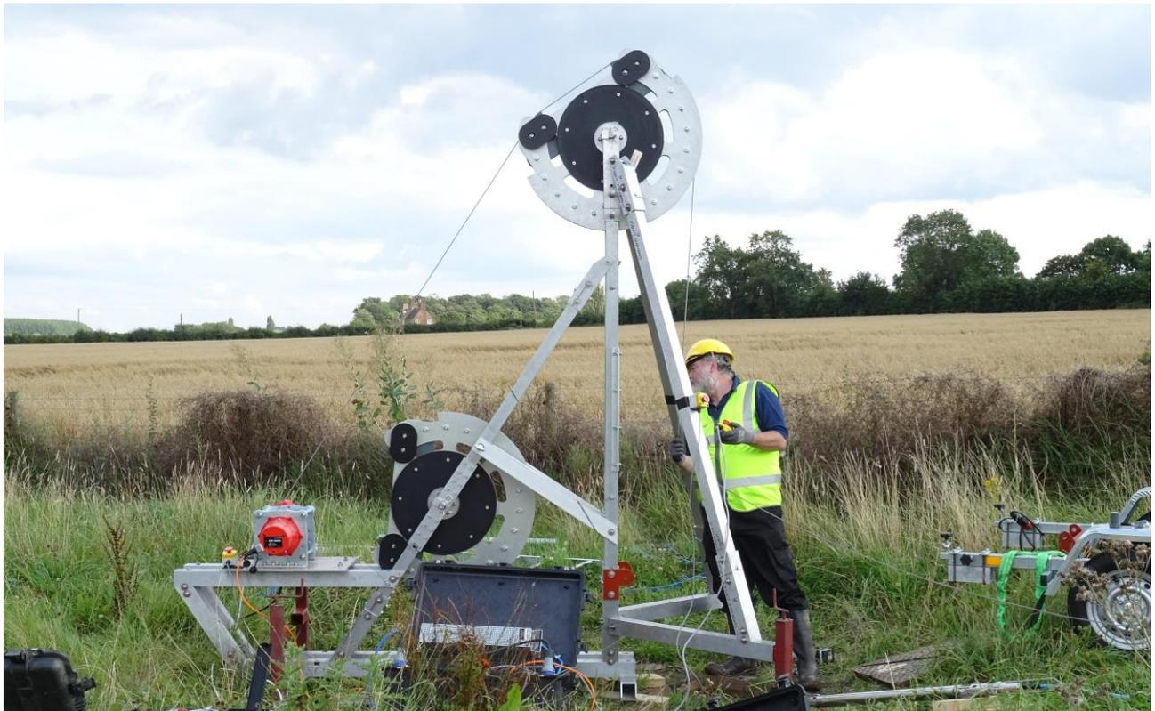
Installing the borehole seismometers at the GeoEnergy Test Bed site near Sutton Bonnington, Nottinghamshire.
